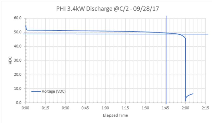
In the discharge curve above, the drop-off below 49 Vdc is very fast. Even with an increased LBCO setting between 49-50 Vdc, it may still not prevent a dead battery condition. The LBCO function only shuts down after a delay of approximately five minutes.
