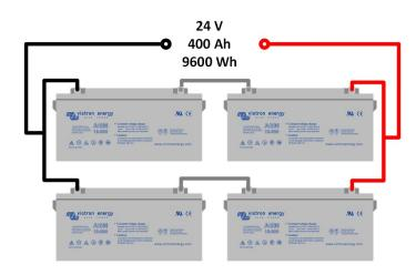
Four batteries in series/parallel
