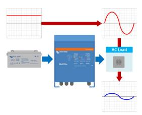
3. This AC current causes (via the inverter) a fluctuating DC current on the battery.
