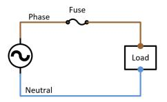
Traditionally, a fuse contains a wire that melts when unacceptable current passes through. As soon as the wire in the fuse has melted the electrical circuit has been broken and no additional current will flow.
