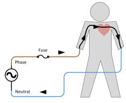
Electric circuit is closed Electricity will flow
