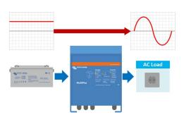
2. The load connected to the inverter creates an AC current in the inverter.
