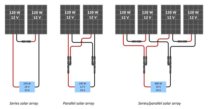
To determine the total power of a solar array, you will simply have to add the power of each module no matter if they are connected in parallel or in series.
