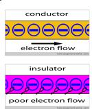
Each material has its own specific resistance. It is measured in  $\Omega$ .m. and the symbol is  $\rho$  (rho).
