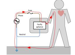
To make electrical installations safer the earth conductor was introduced. The earth wire connects the metal housing to earth.
