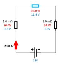
It is important to keep this voltage drop as low as possible. The obvious way to do that is to increase the thickness of the cable or to keep the cable length as short as possible. But there is something else you can do, and this is to increase the circuit's voltage. The cable voltage drop varies for different battery (system) voltages. Generally speaking, the higher the circuits voltage the lower the voltage drop will be.
