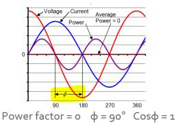
When the power factor is known the apparent power can be calculated.
