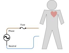
Electric circuit not closed Electricity cannot flow
