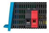
Strip a sufficient length of cable insulation before inserting the bare end into the connector cavity. Avoid cable insulation entering the connector. This can lead to too much resistance and the connector will heat up and potentially melt. Avoid uninsulated cable (bare cable) to be visible outside the connector. This is dangerous it can cause electrocution or a short circuit.
