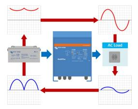
The DC voltage will keep going up and down and is not constant anymore. It now is fluctuating. It will go up and down 100 times per second (100 Hz). The amount the DC voltage fluctuation is called ripple voltage.
