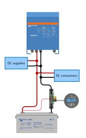
To fix this, move the shunt away from the positive cable (not ideal). Or consider not using shunt at all but use smart batteries that generate their own state of charge.
