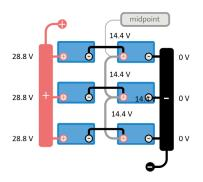
Once the midpoint of the battery bank is connected one battery balancer can be used, instead of using 3 battery balancers (one for each string). Also, a single BMV can be used for midpoint monitoring of the entire battery bank.
