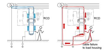
Earth leakage detection can only take place in systems where the neutral conductor is connected to the earth conductor; like in a TN or TT system. Earth leakage detection is not possible in an IT network.
