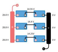
Once each string voltage is equal the midpoints can be connected. Make sure that the midpoint cabling is able to carry the full current between the batteries.
