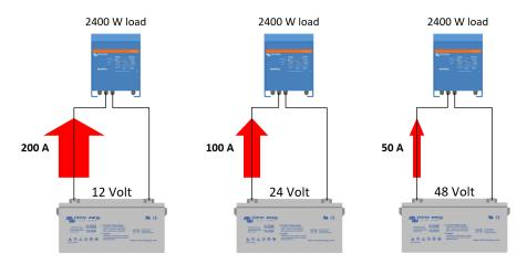
Also, as explained already, a cable has a certain amount of resistance. The cable is part of the electrical circuit and can be treated as a resistor.
