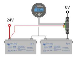
The BMV 702 and BMV 712 have a second voltage input that can be used for midpoint monitoring. It can be wired to the midpoint of the battery bank. The BMV will display the difference between the two voltages or as a percentage. For more info see the battery monitor <u>product page</u>.
