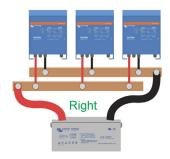
When using busbars, it is in most cases necessary to shield the busbar, especially if the busbar is out in the open. This to prevent people touching the busbar, or to prevent a short circuit if a metal object should accidentally fall across the positive and negative busbars and accidentally short circuit both busbars. An easy way to do this is to mount a Perspex sheet in front or over the busbar. See image on the right.
