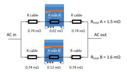
To safeguard against this issue, it is recommended to use long AC, cables of similar length. Always follow the recommended cable lengths and thicknesses as listed in the product manual. Do not increase the cross-section of the AC cabling more than is recommended in the manual!
