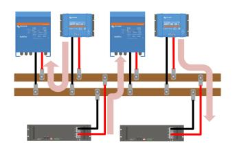
When wiring, make sure all inverter/chargers have the same cable length. Also, the MPPTs need to have approximately the same cable length. And the same for the batteries.
