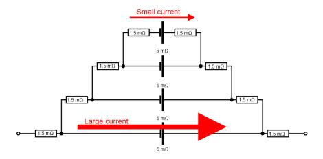
Current will always choose the path of least resistance. Most of the current will therefor travel through the bottom battery. And only a small amount of current will travel through the top battery.
