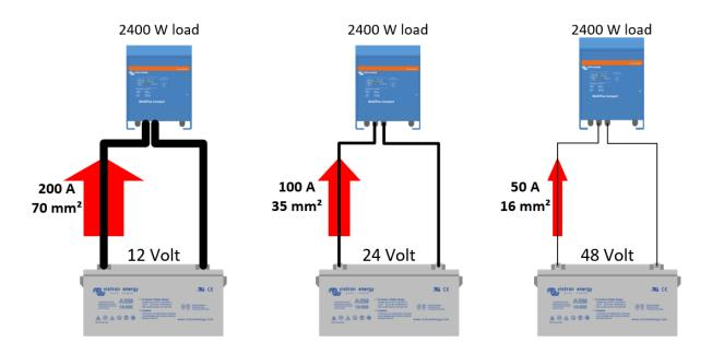
In order to avoid very thick cables, the first thing you should consider is to increase the system voltage. A system with a large inverter will cause large DC currents. If the DC system voltage is increased, the DC current will drop, and the cables can be thinner. The preferred upper inverter power limits per system voltage are:
