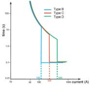
When a short circuit current occurs, with sufficient current, the MCB (B,C or D) is switched off within 100 ms.
