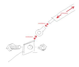
Resistance will be added to the electrical circuit each time a connection is made, or something is placed in the path between the battery and the inverter.
