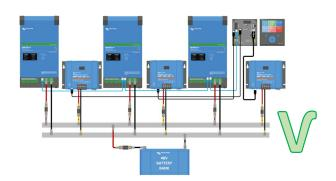
If the system has only one battery bank you should connect the battery bank in the middle of the busbars. But in case of several parallel battery banks or smart batteries, they should also be distributed evenly along the busbars.
