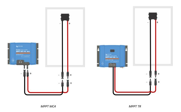
In some occasions the solar panel does not have cables attached. You will then need to attach these yourself. To do this, open the junction box at the rear of the panel and connect the cables there. You can either use solar cables with or without MC 4 connectors. If you are wiring the solar panel directly to the MPPT, then this is what the installation will look like:
