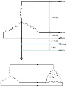
When setting up 3 phase inverter/chargers they will need to be set up in a star configuration. They need to have a common neutral. Delta is not allowed. But the 3-phase inverter/charger system can power a "delta" configured load.
