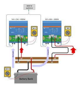
To achieve a balanced system, you will need to use the same cable type, cross-section and cable length to each unit from the battery bank or from the busbars. Also ensure that all cable lugs are identical, and all connections are tightened with the same torque values. Consider using busbars or power-posts between the battery bank and the inverter/chargers.
