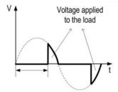
These often are loads that contain semiconductors, like diodes or LEDs. Examples of these are AC LED lighting, light dimmers, heat guns and certain soft start devices. When an inverter powers a non-linear load, it will go earlier into overload than the power rating of the load.
