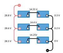
First make sure that each string has the same voltages by using a common negative and positive connection point or busbar.
