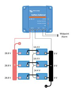
But please be aware, that the only reason to use the midpoints of a battery bank is for balancing and/or monitoring purposes. It is not allowed to connect loads to the midpoint of a battery bank in order to be able to run loads that require a lower voltage. Doing so will create a large imbalance in a battery bank. This imbalance is much bigger than a battery balancer can potentially rectify (larger than 0.7 A) and the battery that is used to provide the lower voltage will fail prematurely.
